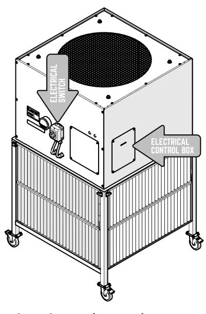
When the equipment is powered on, a light is emitted behind the frosted pane of the front access panel of the electrical control box.
