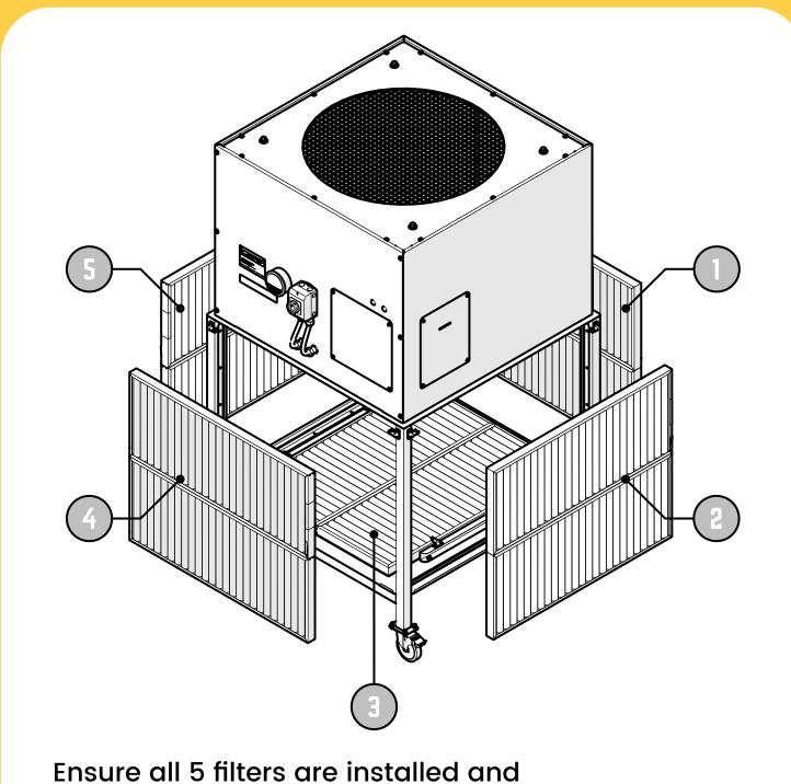
correctly oriented. Particulate will be captured on the side facing out.
